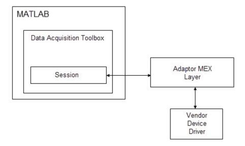
Hardware drivers are provided by the device vendor. For example, to acquire data using a National Instruments® board, the appropriate version of the driver must be installed on your system. Hardware drivers are not installed as part of the toolbox, but a suitable driver is usually installed on PCs that are equipped with a sound card. For any other devices, the drivers must be installed.
