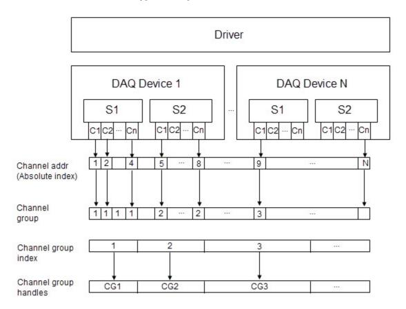
This diagram illustrates the process of enumeration performed during daq.getDevices. Through the driver, the adaptor accesses the numerous supported devices, and determines their subsystems and channels. The adaptor then derives an absolute (unique) index for each channel, and assigns each to a channel group. Each channel group has an index, and a resulting unique channel group handle. Through these handles, the adaptor performs the operations of a data acquisition session.
